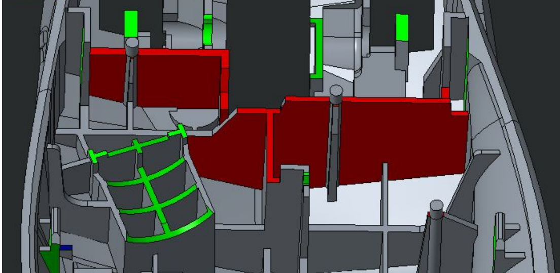
Figure 4: Red parts show noise-dampening ribs inside M330 Silent Plus top case
