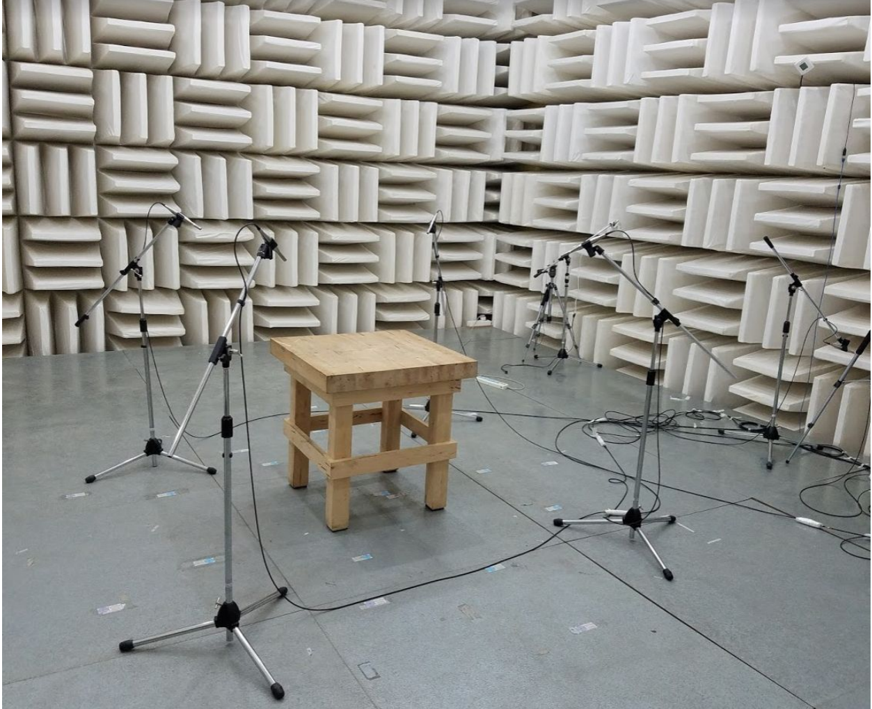
Figure 5: Testing setup at Foxconn CMC anechoic chamber with < 6 dBA background noise
