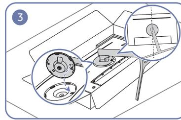
Place the stand neck of the display on the device as per the positions of the fasteners.
